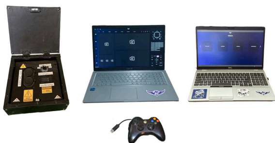
Fig. 21: Orca's Control Station.
