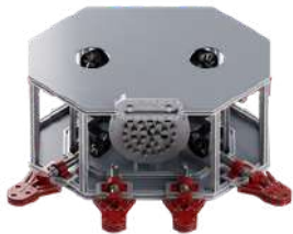
Figure 21: Rejected Initial Frame Design Concept [11] Made by Ahmed Hatim
