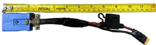
Figure 10: Fuse placement within 30 cm of Anderson Connector Photo by Marwan Mohamed
