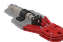
Figure 44: GLACIUS Gripper CAD [11] Made by Yousab Youssef
