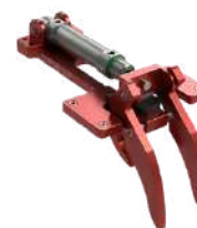
Figure 45: GLACIUS Jaw Gripper CAD [11] Made by Mohamed Youssef
