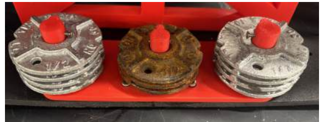
Figure 24: Modular ballast using industrial washers
