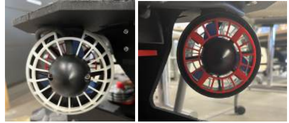
Figure 30: The front (left) and back (right) of a shrouded thruster
