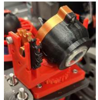
Figure 25: Deepwater Exploration Explore HD 3.0 Camera in Custom Housing
