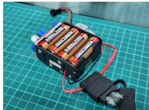
Figure 14. Battery and Fuse
