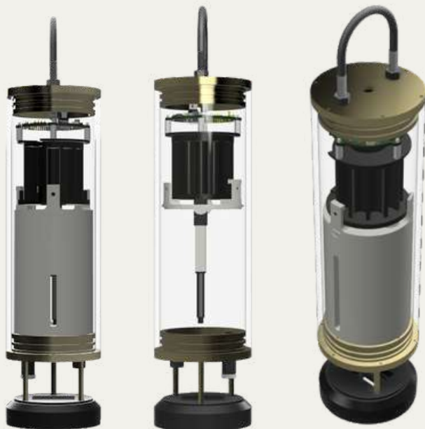
Figure 1. Vertical Profiling Float
