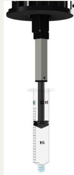
Figure 2. Buoyancy Engine Mechanism
