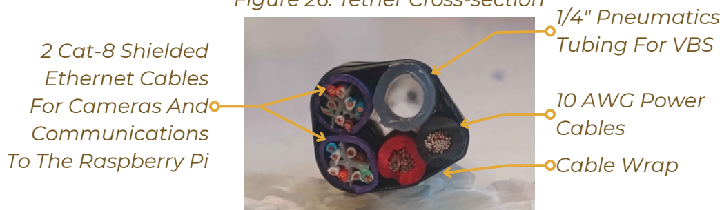
Figure 26. Tether Cross-section
