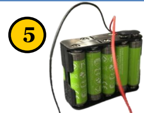
Figure 2. 12 V Battery Pack
