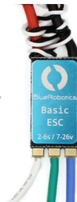
Figure 8: Blue Robotics Electronic Speed Controller, measuring 32 x 17 mm. Credit: Blue Robotics.
