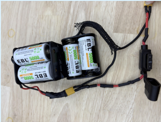
FIGURE 3: AVIVA BATTERY AND FUSE
