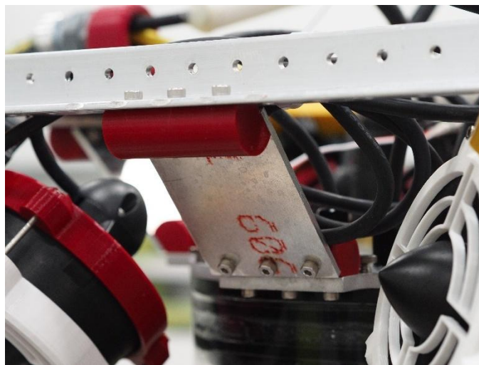
FIGURE 12: DETAIL VIEW OF CUSTOM MOUNT THAT HOLDS ONE END OF THE CANISTER TO CUBERT'S FRAME.
