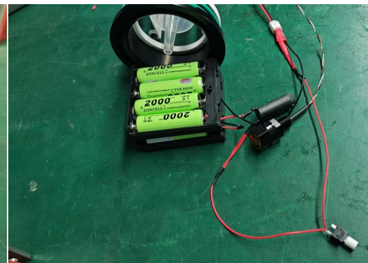
Figure 4. Battery and fuse close up
