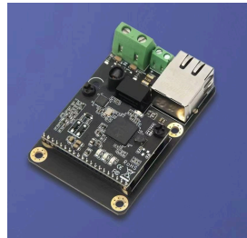
Figure 10: PLC Data Module
