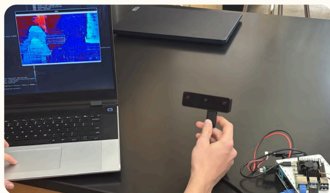
Figure 4 - Stereovision Testing Before Final Integration
