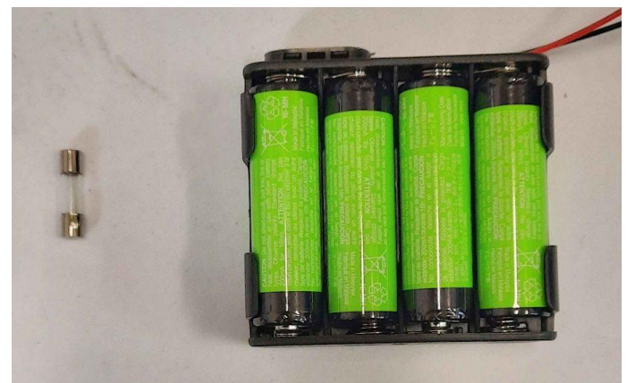
Fig 3. Battery Pack and 2A Fuse
