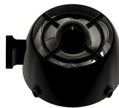
Fig. 18: Thrust housing and toroidal propeller
