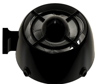
Fig. 27: Fused power connector and propeller shroud
