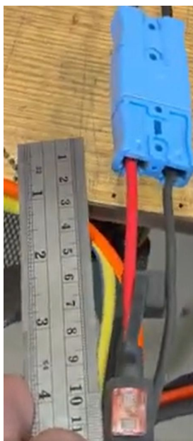
Fig. 27: Fused power connector and propeller shroud
