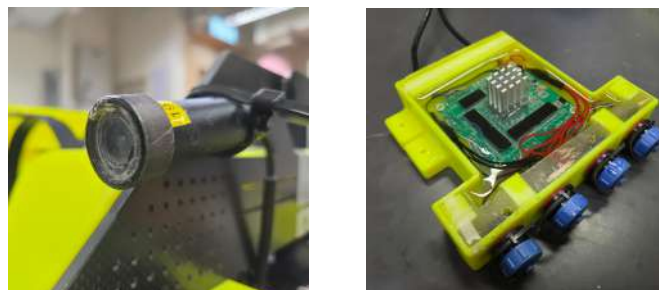
Fig. 16: IP Camera and IP Camera Board
