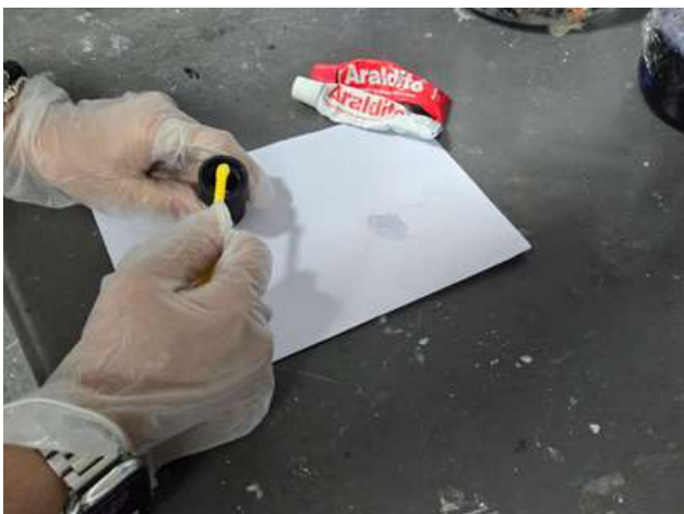
Fig. 58: Wear gloves when using epoxy
