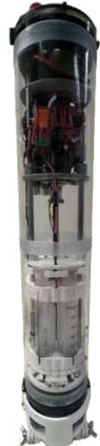
Fig. 56: Real-life buoyancy engine
