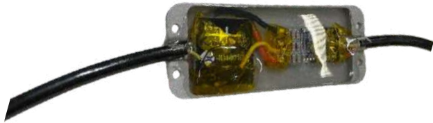
Fig. 27: Water Cooling ESC
