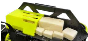
Fig. 20: Buoyancy system of Thunderbolt
