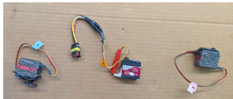
Fig. 32: Three failed servos from previous years advertised as waterproof.
