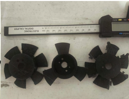
Fig. 26: 3D-printed prototype propellers
