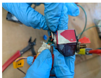
Figure 37: Testing the motor with a 9-V battery (left) Figure 38: Closeup on the inside state of failed servo 3 (right)
