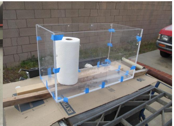
Fig. 27: Mock up of aquarium for testing motors
