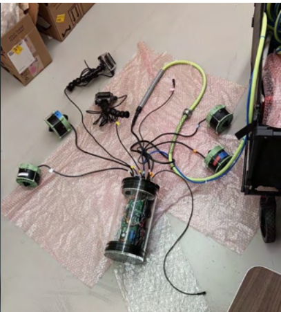
Fig. 30: Frame teardown of ROV for electrical mapping
