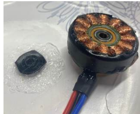
Figure 23: Potting inexpensive motor
