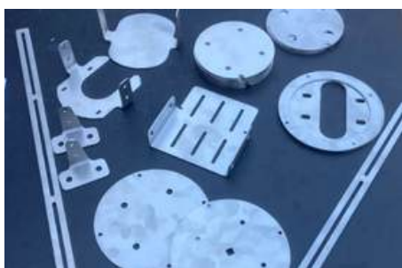
Figure 27: Sheet metal rails, shelves, ballast (left)
