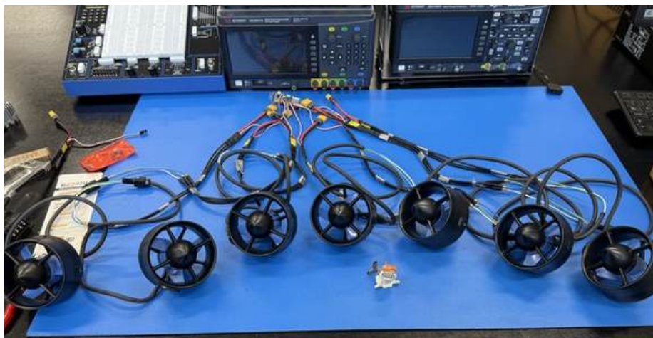
Figure 14: Eight thrusters and ESCs connected to the PWM Expansion Board
