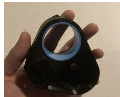
Figure 25: Dry running bearing for wrist shaft
