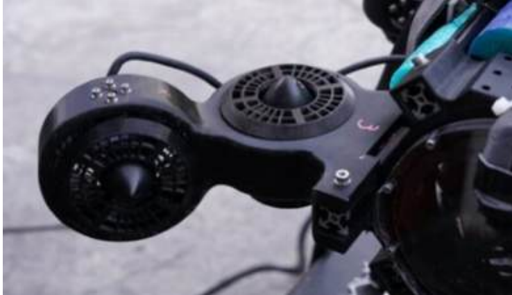
Figure 11: Thruster Mount with T-200 propellers
