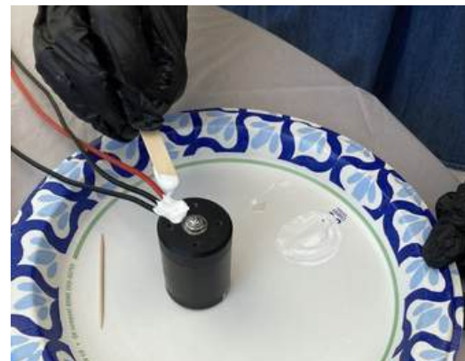
Figure 24: JB Welding DD3130 motor
