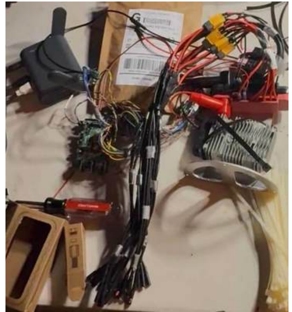
Figure 15: The Internal electronics of the ROV connected to the WiFi router
