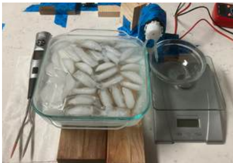
Figure 38: Peristaltic pump feasibility testing
