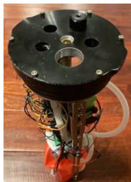
Figure 27: Sheet metal rails, shelves, ballast (left)
