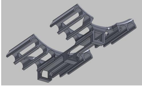
Figure 18: The ballast frame and C-shaped cups.
