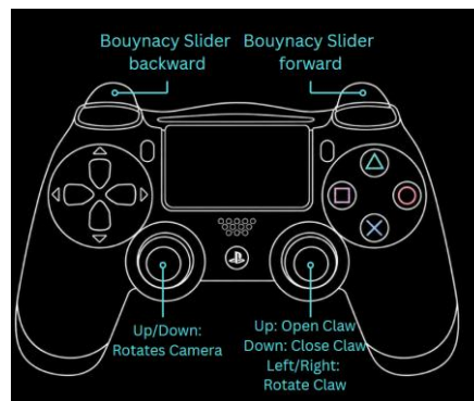
Figure 11: Diagram of Human Input Manipulator Controller.
