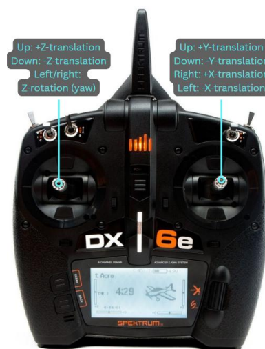
Figure 12: Diagram of Human-Input ROV Controller.
