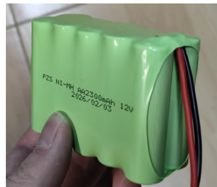
Figure 4: NiMH Battery Pack
