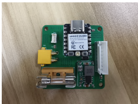
Figure 5: Custom control and drive PCB with XT30 power connectors
