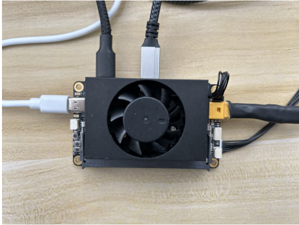
Fig. 6. Physical view of the Jetson Orin NX.
