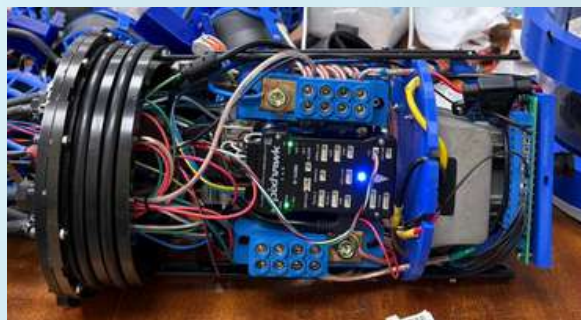
Figure 9: Internal electronics enclosure demonstrating strict wire segregation
