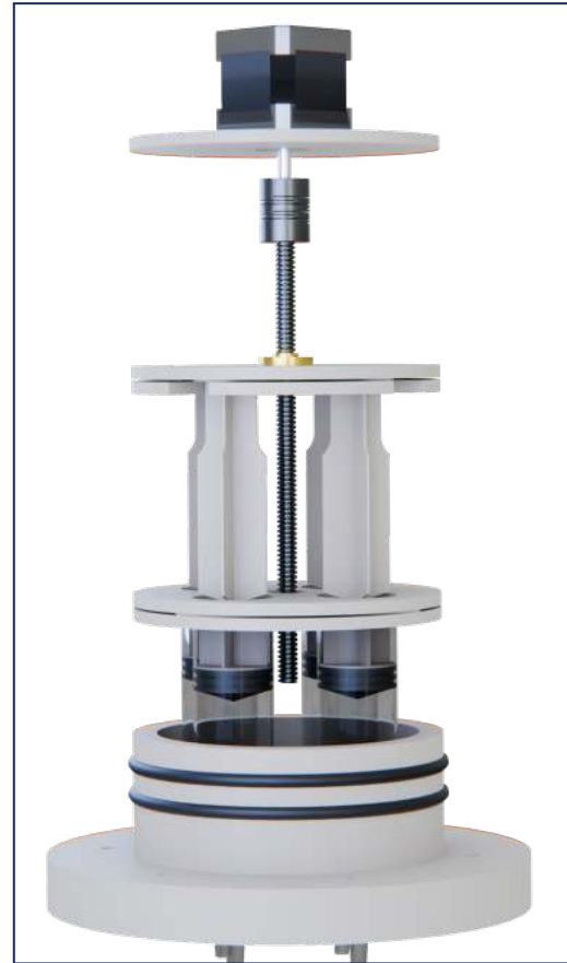
Figure (2): Clarification of the buoyancy engine mechanism
