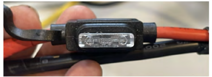
Figure 22: The 25A fuse
