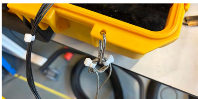
Figure 12: Strain-relief design of Groundstation
