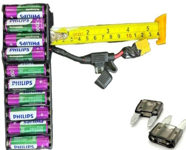
Figure 5 Battery pack used and in line 2 amp fuse installed
