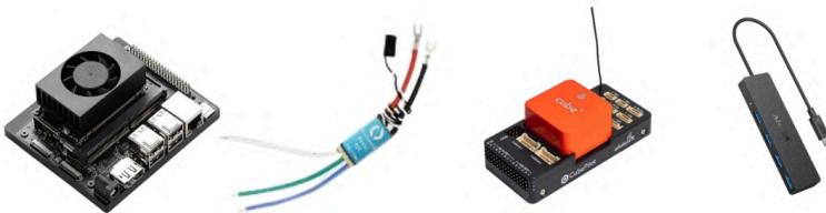
Fig 11: Electrical components; Left to right: NVIDIA Jetson Orin Super nano | ESC | Cube flight controller | Anker USB hub
