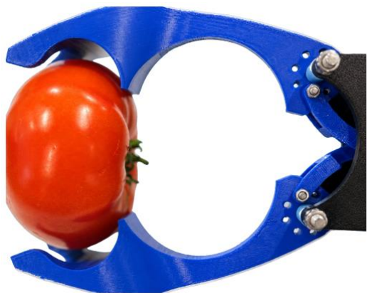
Figure 12: Testing Triton's grippers for safety by limiting pneumatic pressure and bore size based on testing on tomatoes. Photo by M. Lipson
