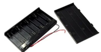
Figure 4: 12-volt Independent Power Source
