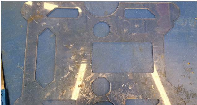
Figure 5: Lexan Plastic Frame
