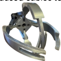
Figure 38: Prototype of claw design - Photo by Robert McIntosh
