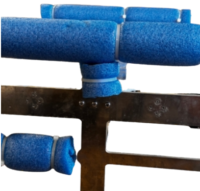
Figure 11: Pool noodles on ROV- Photo by Piper McGuire-Turcotte
