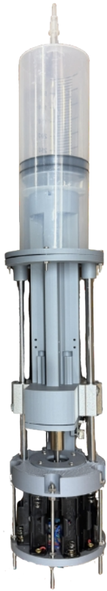
Figure 35: Vertical Profiling Float Interior- Photo by Robert McIntosh.
