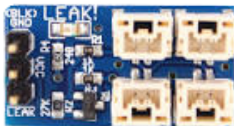
Figure 31: Leak detector that is inside of the enclosure to detect water - Photo by Blue Robotics
