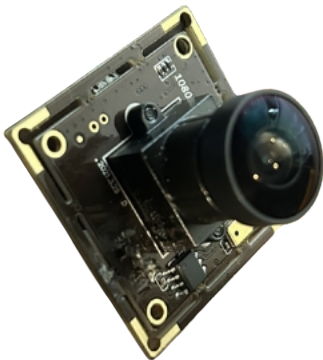
Figure 19: The Sony IMX323 used in enclosure - Photo by Matthew Schwarting
