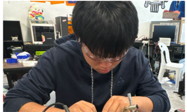
Evan preparing the control box wires to be soldered Photo taken by: Selena Tan
