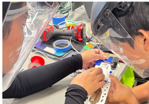
Evan and Yuchen using the soldering iron to weld together the 3D printed claw screws. Photo by: Selena Tan
