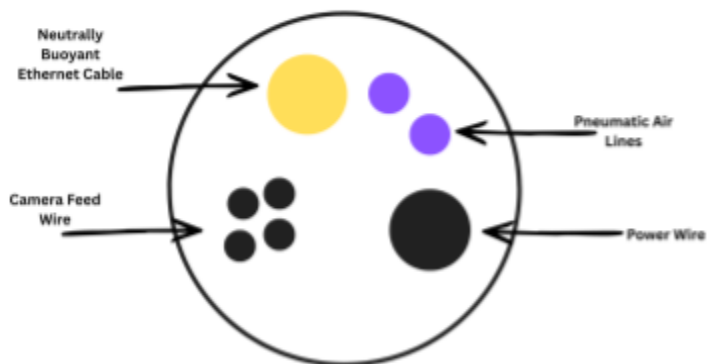
Figure 8: Cross section of the tether- Made by Belle Gibbons
