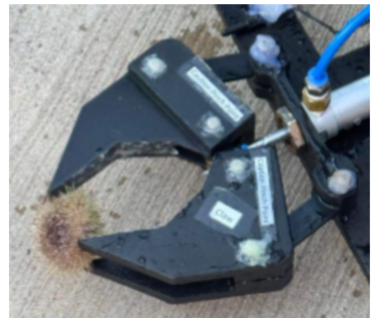
Figure 11: Image of the pneumatic claw in action | Photo taken by Marcus Flynn
