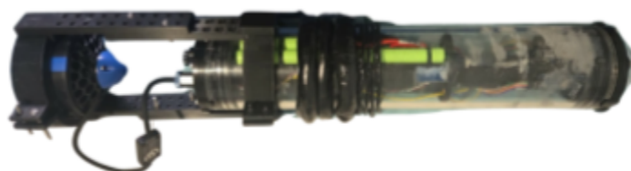
Figure 15: Shark Fin Vertical Profiling Float - Image by Jerry Cabot
