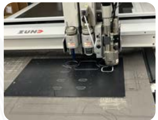
MUREX ROV Chassis Plate CNCing. Photo: O. Chang
