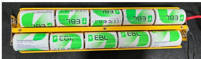
Figure 19: NiMH eco-friendly batteries within company-made float battery case Taken by Sophia Zhang
