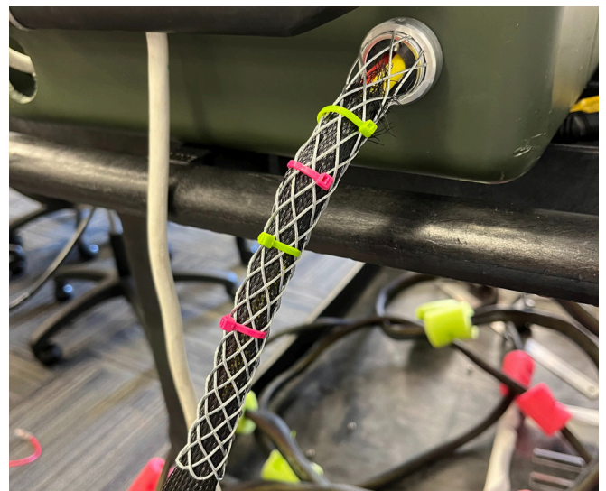
Figure 31: Nautilus's topside strain relief Taken by Anya Li
