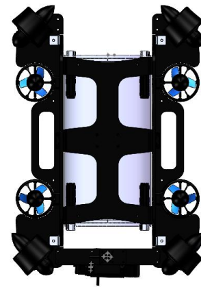
Figure 11: 8-Thruster Vector Propulsion System Layout of ROV
