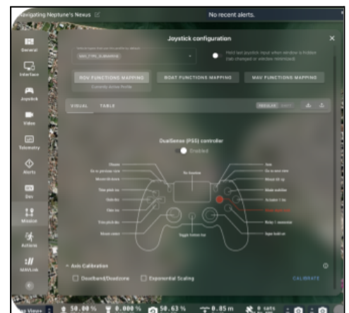
Fig 13: Controller Configuration on Cockpit
