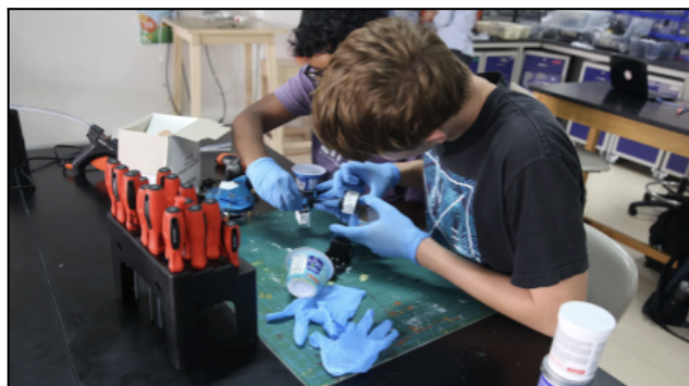
Fig 30: Servo Waterproofing Process with appropriate PPE Credit: Ronan Erickson
