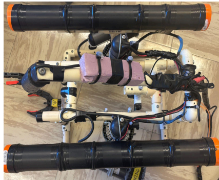
Diagram 5. Bird's eye view of Bonabot and its buoyancy. - Photo by Jacinda Elson
