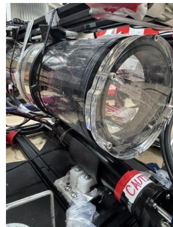
Figure 6: Photo of Watertight Enclosure
