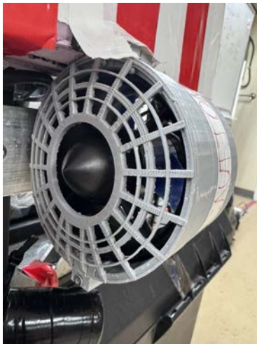
Figure 19: Photo of Waldo T200 Thruster Photo taken by: Taara Gill
