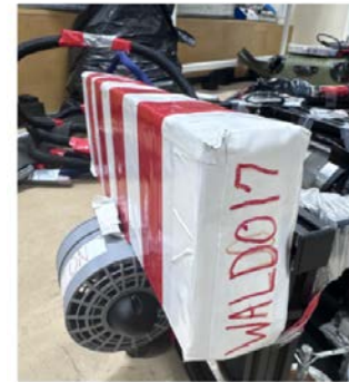
Figure 11 & 12: Photos of Waldo XVII's Buoyancy System Photo Taken by: Taara Gill
