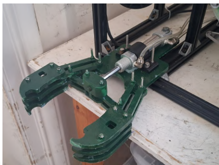
Fig. 14. Leviathon's pneumatic HDPE gripper in an open position. Photograph by Hour Ahmed.
