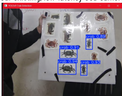
Fig. 22. Our custom YOLO model detecting invasive crabs during training. Image captured by Ammar Abdelhakam.
