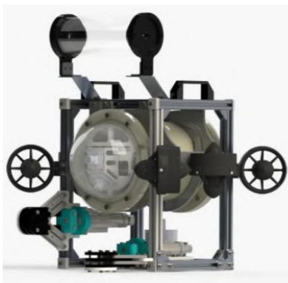
Fig. 5. SolidWorks CAD render of Kratos, our previous ROV. Render created by Hour Ahmed.
