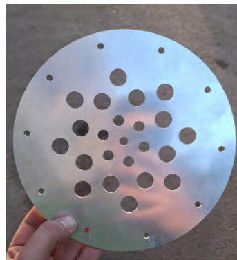
Fig. 13. Custom laser-machined rear aluminum face. Photograph by Eyad Wagdy.
