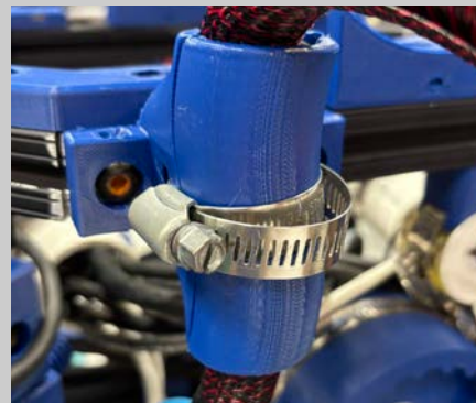
Figure 10, ROV-Side Strain Relief: The strain relief design on the ROV by Cameron Bell. (Aiden Bunning)
