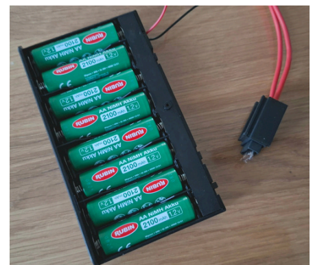
Figure 2: NiMH Battery Pack and Fuse
