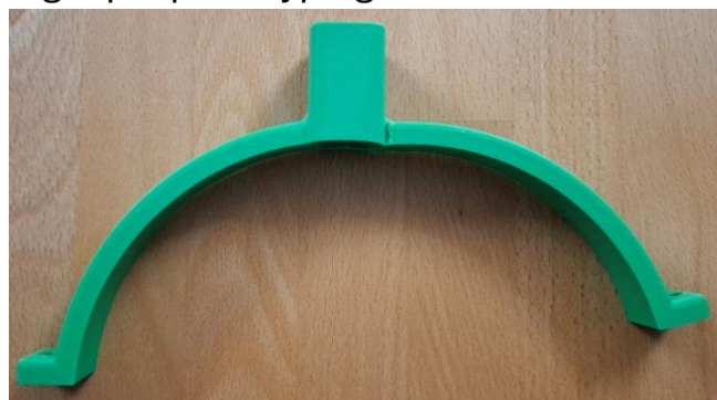
Figure 4: Design iteration with structural failure - Photo taken by Florian Theile
