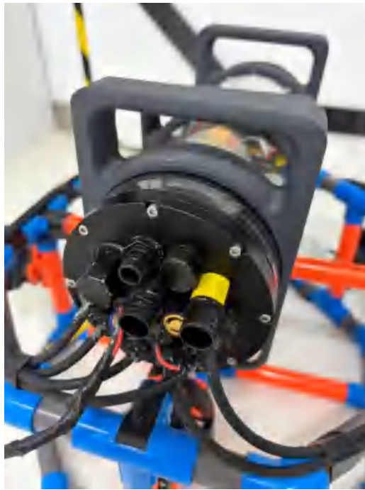
FIGURE 40: WATERPROOF OF THE SEALED CABIN
