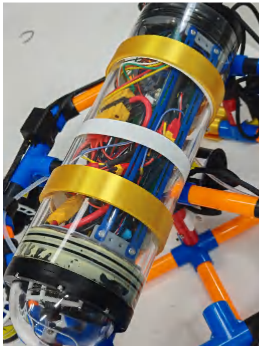
FIGURE 41: THE FASTENERS OF THE 3D-PRINTED SEALED CABIN
