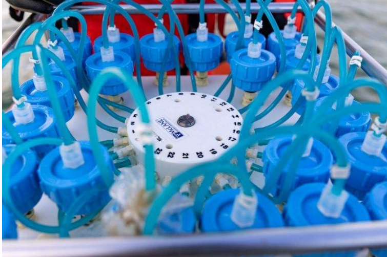
An eDNA sensor. Detecting fish with the innovative Fish Sensing Box
