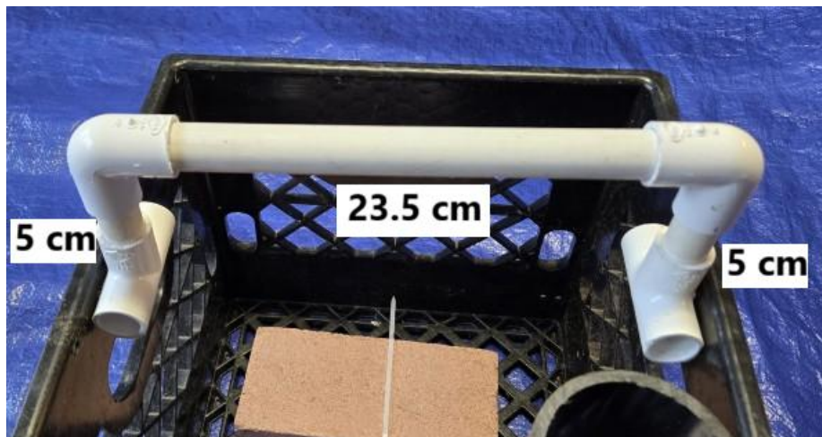
The lobster pot can be lifted by the 1/2-inch PVC pipe, which is screwed into the milk crate.
