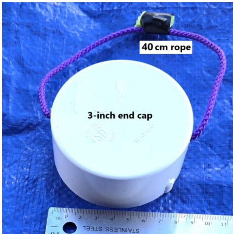
The cover of the oil platform port is constructed from a 3-inch PVC end cap . A 40 cm length of rope acts as a carrying mechanism for the cover. The oil platform port cover is considered debris; companies must return the cover to the surface, side of the pool or it must be under control of their ROV at the end of the product demonstration run.
