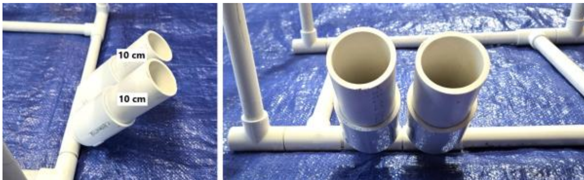
The Holyrood subsea observatory connection port is constructed from 10 cm lengths of 1 1/2-inch PVC pipe, 1 1/2-inch couplings, and 1 1/2-inch to 1/2-inch reducer bushings. Left: Side view. Right: Front view.
