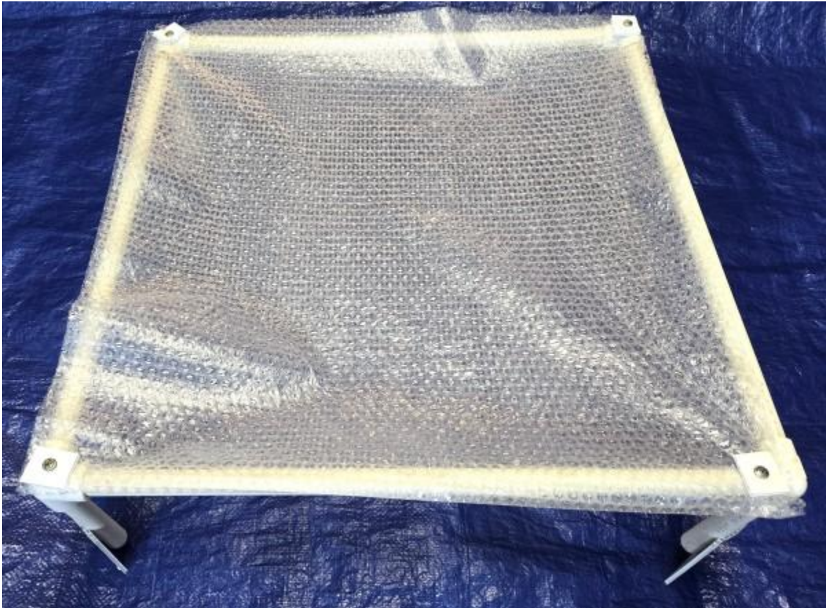
Bubble wrap or clear plastic covers the top of the iceberg. Design note: 2 cm x 2 cm squares of corrugated plastic sheeting will prevent the bubble wrap from tearing when screws are inserted.
