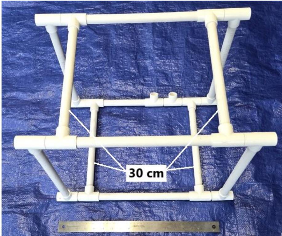
The complete 1/2-inch PVC framework of the Holyrood subsea observatory.
