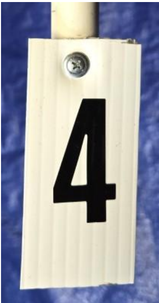
The five survey points around the iceberg will be constructed from 2-inch vinyl numbers on a 10 cm x 5 cm rectangle of corrugated plastic sheeting.
