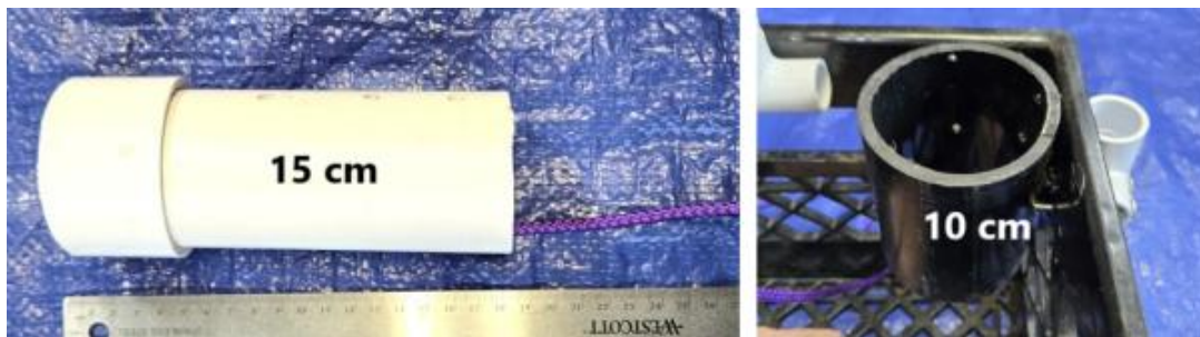
Left: The buoy is constructed from 2-inch PVC pipe and a 2-inch end cap. Flotation inside the pipe makes the buoy positively buoyant. Right: The buoy holder is constructed from 3-inch pipe.
