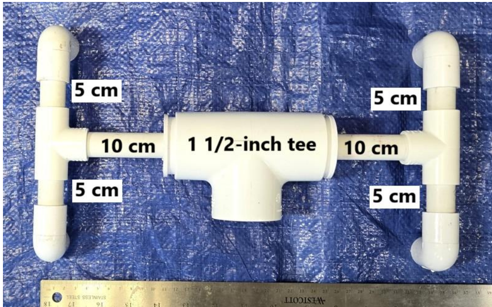
The oil platform port is constructed from 1/2-inch and 1 1/2-inch PVC pipe.
