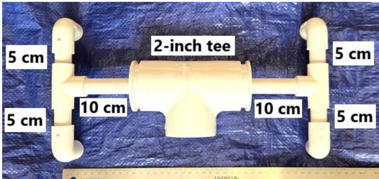
The oil platform port is constructed from ½-inch and 2-inch PVC pipe.
