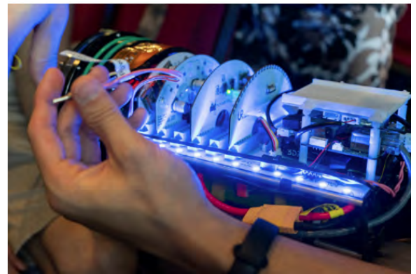
Fig. 42 Backplane with fail-safe system and LED display
