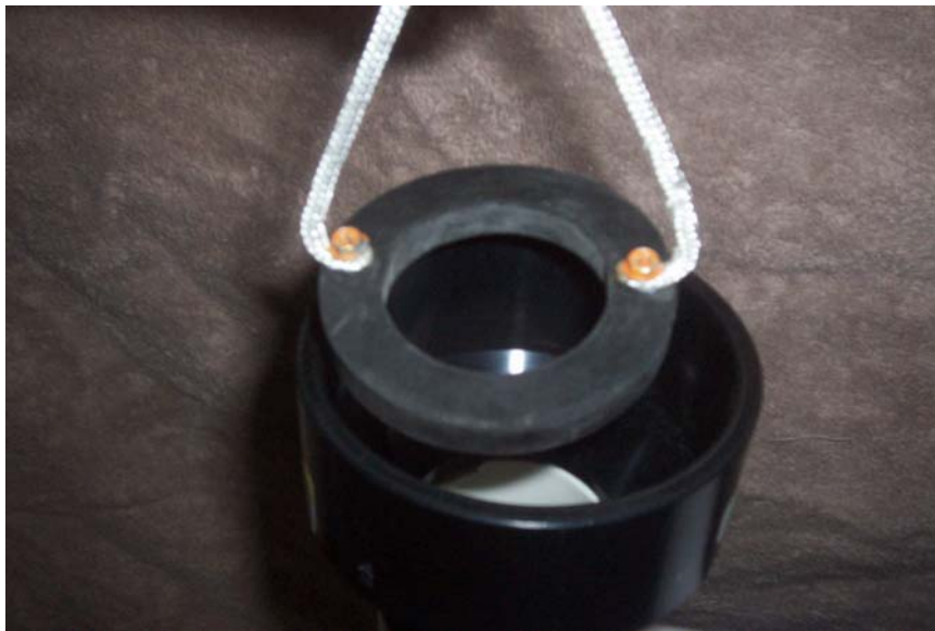
Gasket being inserted into well head
