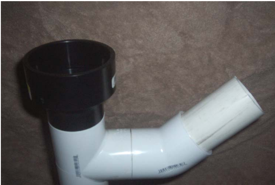
Wellhead without cover
