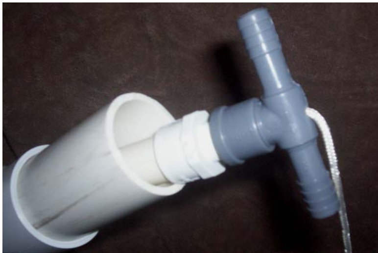
Hot stab inserted into port
