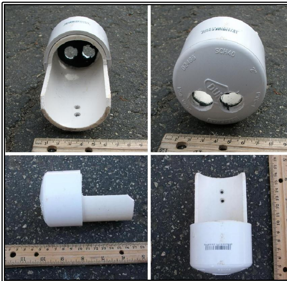
RANGER mission photo #12: Front view, rear view, side view, and top view of CTA bulkhead connector.
