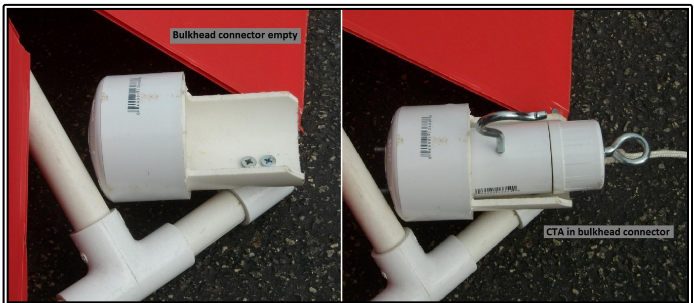
RANGER mission photo #14: CTA bulkhead connector on BIA without and with CTA connector installed.
