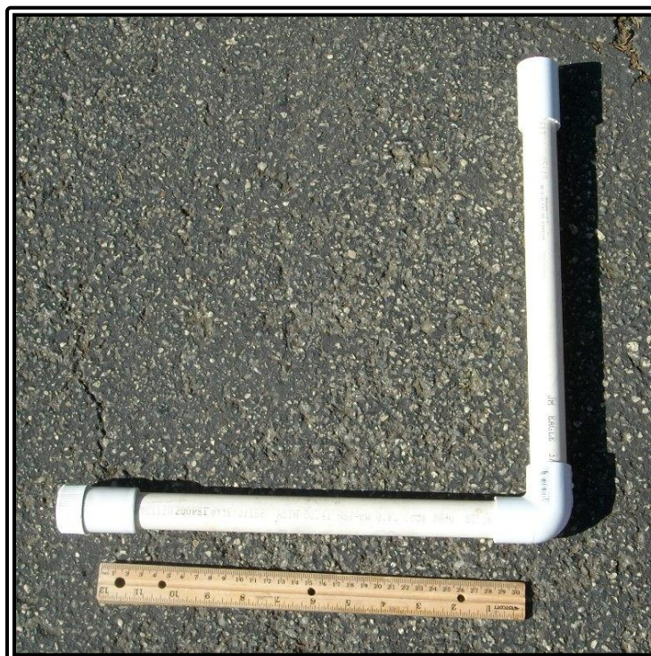
RANGER mission photo #24: 3/4-inch PVC pipe inside the vent structure.
