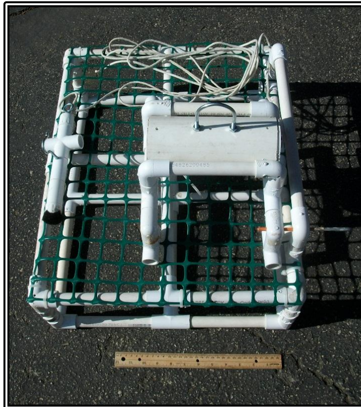
RANGER mission photo #20: Side view of elevator with OBS, OBS cable connector, and cable.
