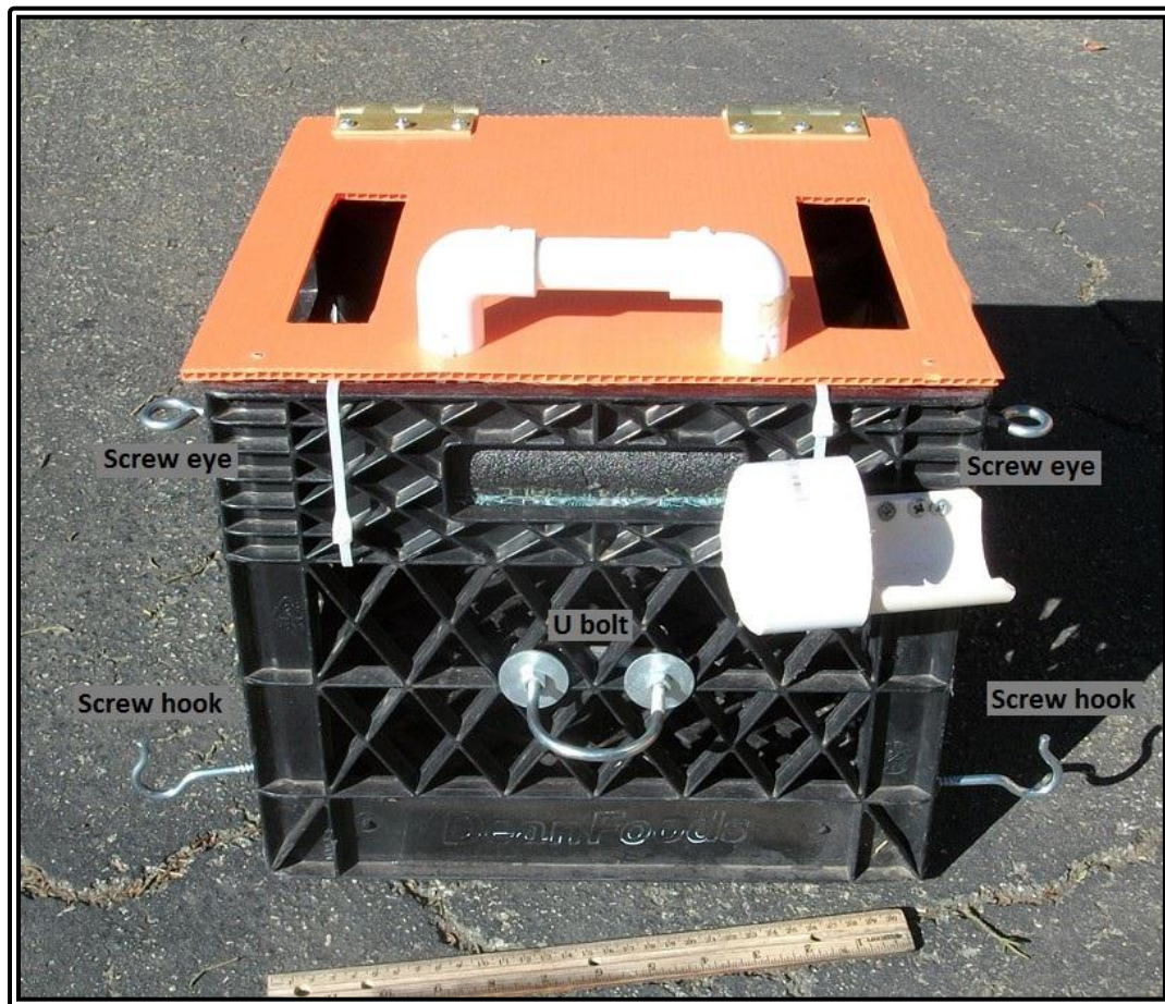
RANGER mission photo #28: Grab points on mooring platform.
