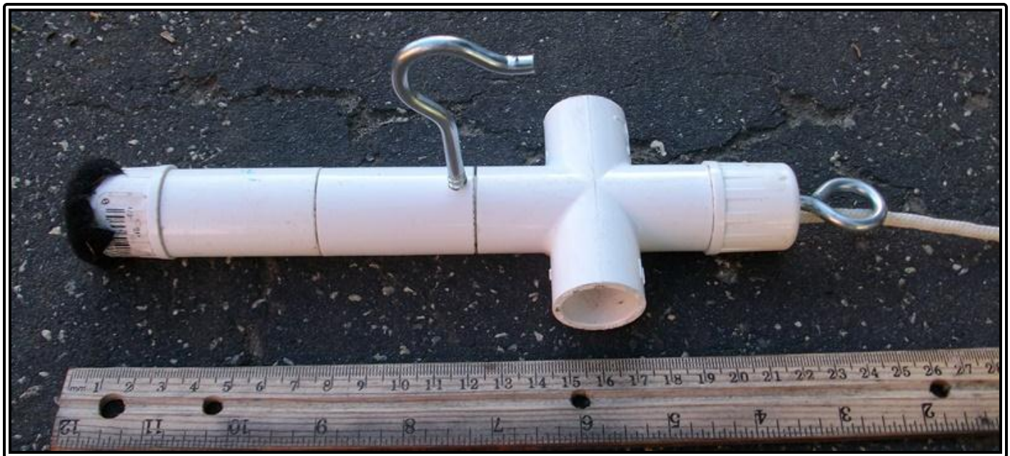
RANGER mission photo #18: OBS cable connector.
