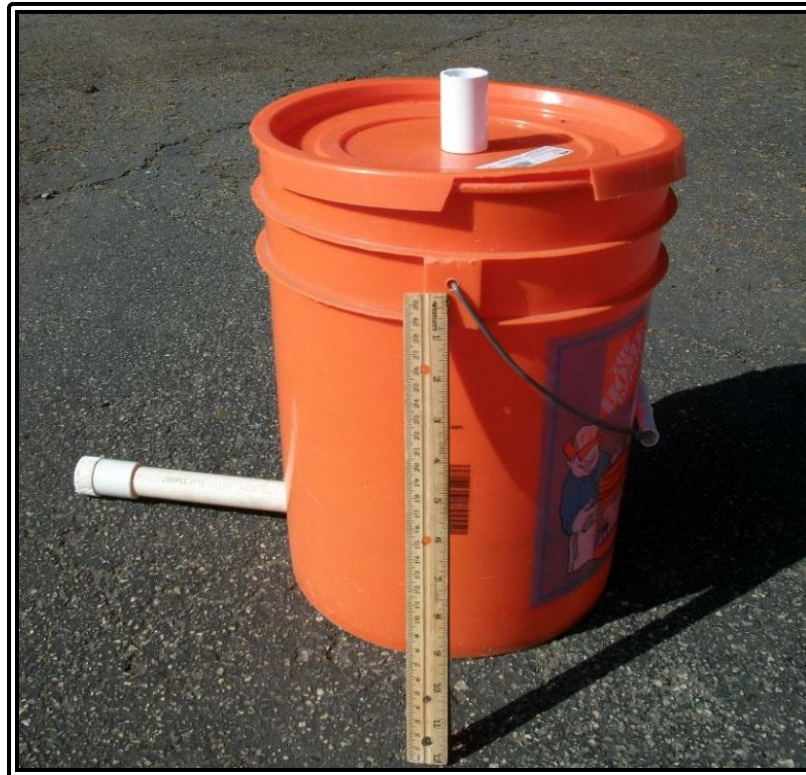
RANGER mission photo #23: Vent structure (5-gallon bucket).
