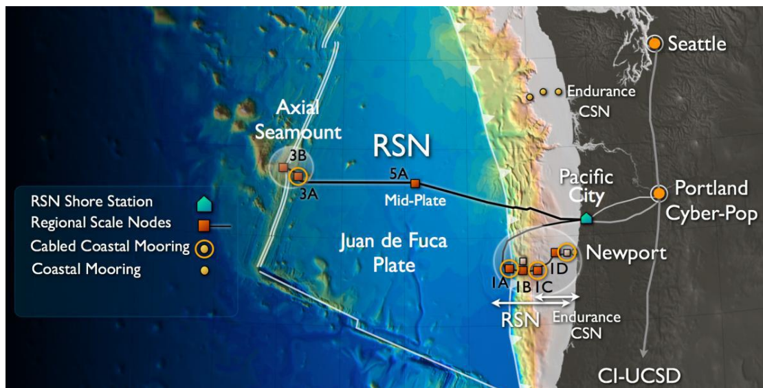
The RSN primary infrastructure, showing the location of the primary nodes
