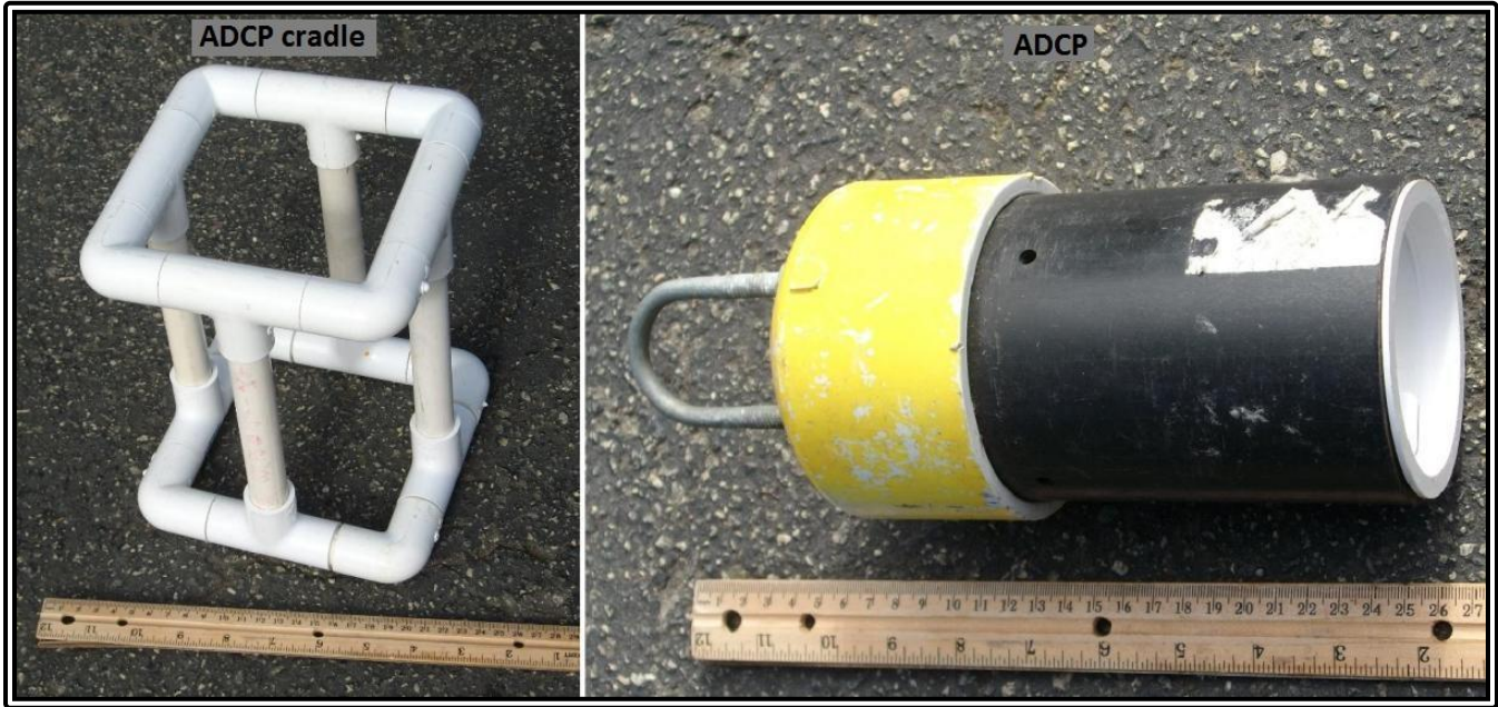
RANGER mission photo #29: ADCP cradle and ADCP.
