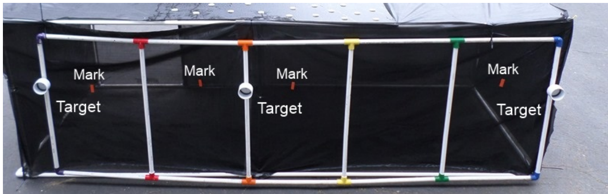
EXPLORER build photo #30: Three “scan” targets attached to the photomosaic grid.
