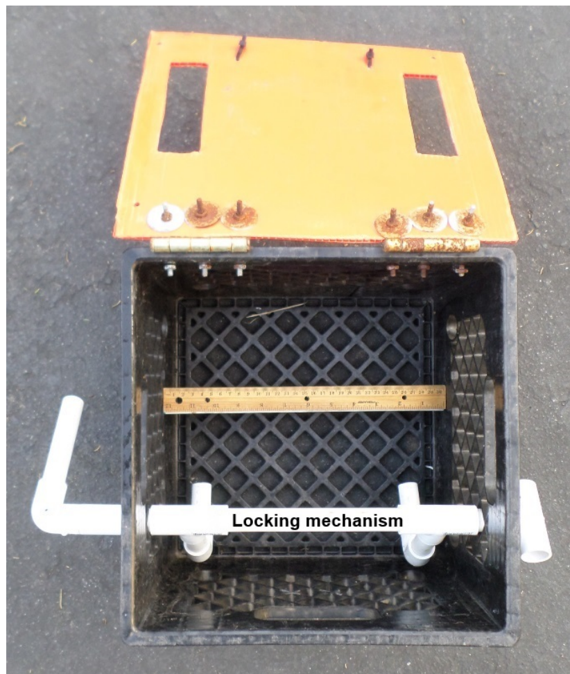
EXPLORER build photo #33: Locking mechanism inside the milk crate.
